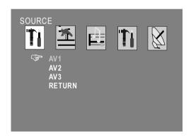
When screen appears "SOURCE" Press Menu button (1) to enter video signal input selection. [The symbol show current video input.]
